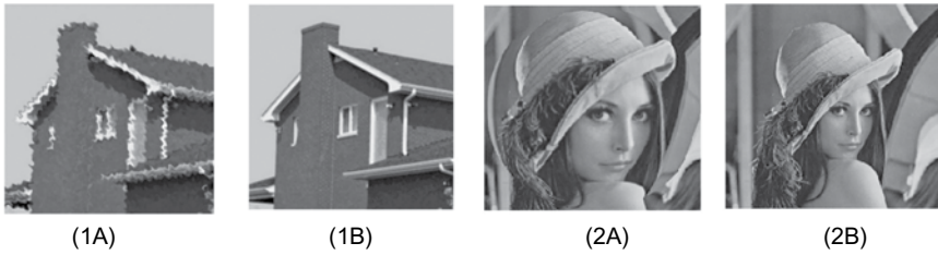
FIGURE 1.7 (1A) Ripple effect, (1B) Nonlinear correction output, (2A) Spherical effect, and (2B) Nonlinear correction output.
