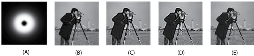
FIGURE 4.21 (A) Image of BBP filter, (B) Original image, (C) Output of BBP filter ( F_L = 30, F_H = 50 ), (D) Output of BBP filter ( F_L = 30, F_H = 150 ), and (E) Output of BBP filter ( F_L = 70, F_H = 200 ).
