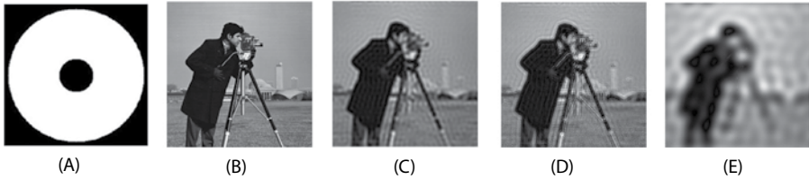
FIGURE 4.20 (A) Image of IBP filter, (B) Original image, (C) Output of IBP filter ( F_L = 30, F_H = 100 ), (D) Output of IBP filter ( F_L = 30, F_H = 50 ), and (E) Output of IBP filter ( F_L = 10, F_H = 90 ).
